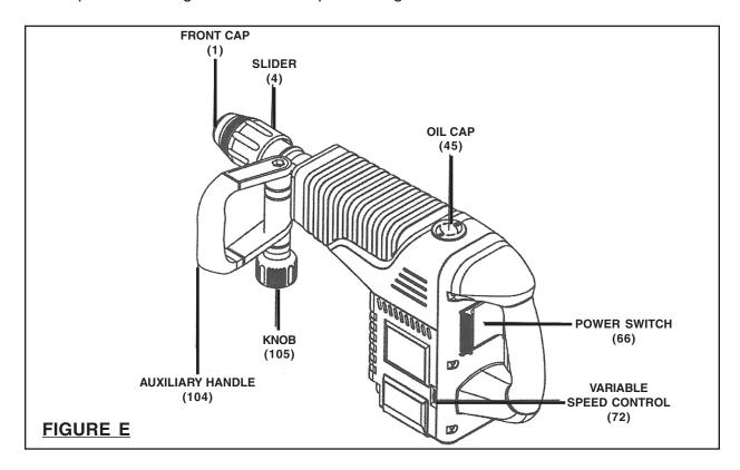
Oil Cap (45): Prior to the Demolition Hammer's first use, remove the Oil Cap and check to make sure the tool is properly filled with grease. If necessary, fill the tool with approximately 1-1/4 ounces of #3 Lithium-based grease (not included). Then, replace the Oil Cap. Thereafter, replace the grease at the end of every 70 to 80 hours of tool use. (See Figure E.)
